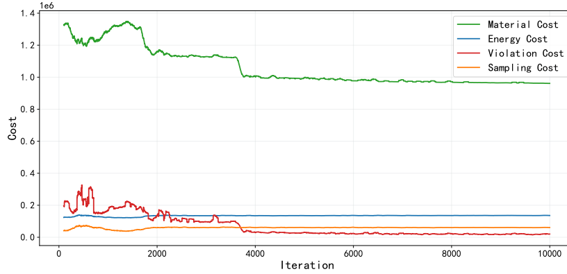
Figure 5: Cost component evolution during training. Material and violation costs decline after initial exploration, while energy and sampling costs remain stable.
